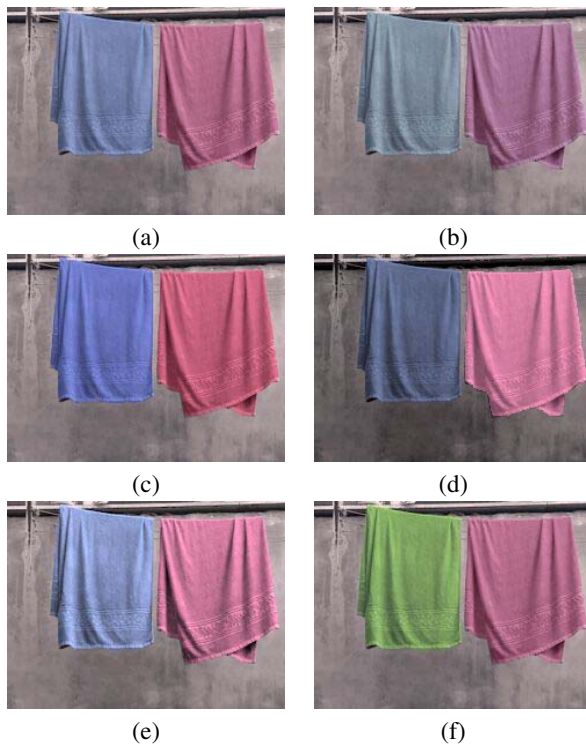
Figure 12: (a) Original image (segmented into 3 color lines). (b) Decreasing the color saturation. (c) Increasing the color saturation. (d) Shifting the intensities making one object brighter and the others darker. (e) Stretching the lines. (f) Changing colors.
