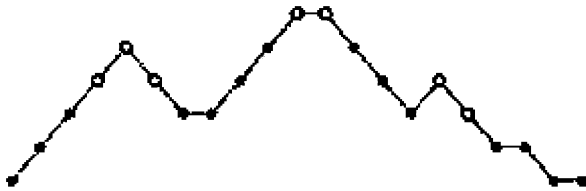
Fig. 2. Under five-point profile-recognition criterion, empty circles are picked as possible ridge points.
