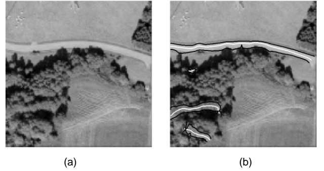
Fig. 9. Lines and their width detected (b) in an aerial image (a).
